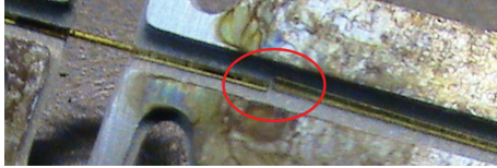
FIGURE 11: Fiber break at one end of the Bragg grating in the FBG_1 sensor.
