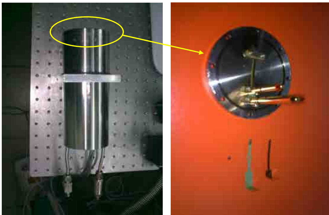
Figure 2.7. R. M. Jordan stainless steel pulsed valve.
