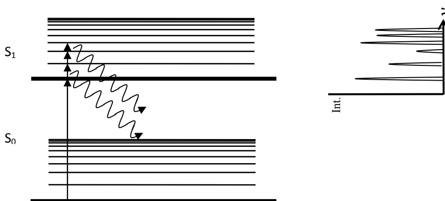
Figure 3.1. Diagram of a LIF experiment under collision free conditions. The laser ( h\nu ) excites the system from the ground state to the vibronic levels of the excited state, while the total fluorescent emission is recorded as a function of the laser wavelength.
