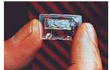
Lehenengo zirkuitu integratua Jack S. Kilby 1958ko udan (Courtesy of Texas Instruments)
