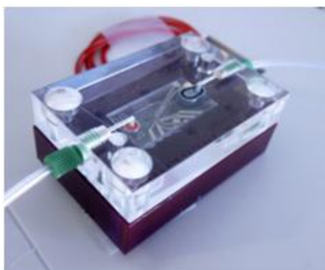
Figure 6.3. Image of the packaging with an LFCS device, which provides connection to all source and control elements.
