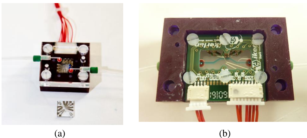
Figure 5.4. Packaging used for the characterization of the micro flow sensor, enabling different dye dimensions of (a) 1 \times 1 \text{ cm}^2 and (b) 2 \times 1 \text{ cm}^2 . The chip holder has electric connections made with spring loaded pins inserted in a printed circuit board (PCB). The bottom methacrylate has threaded fluidic connectors (Upchurch Scientific®) and O-rings to ensure leak tight seal.
