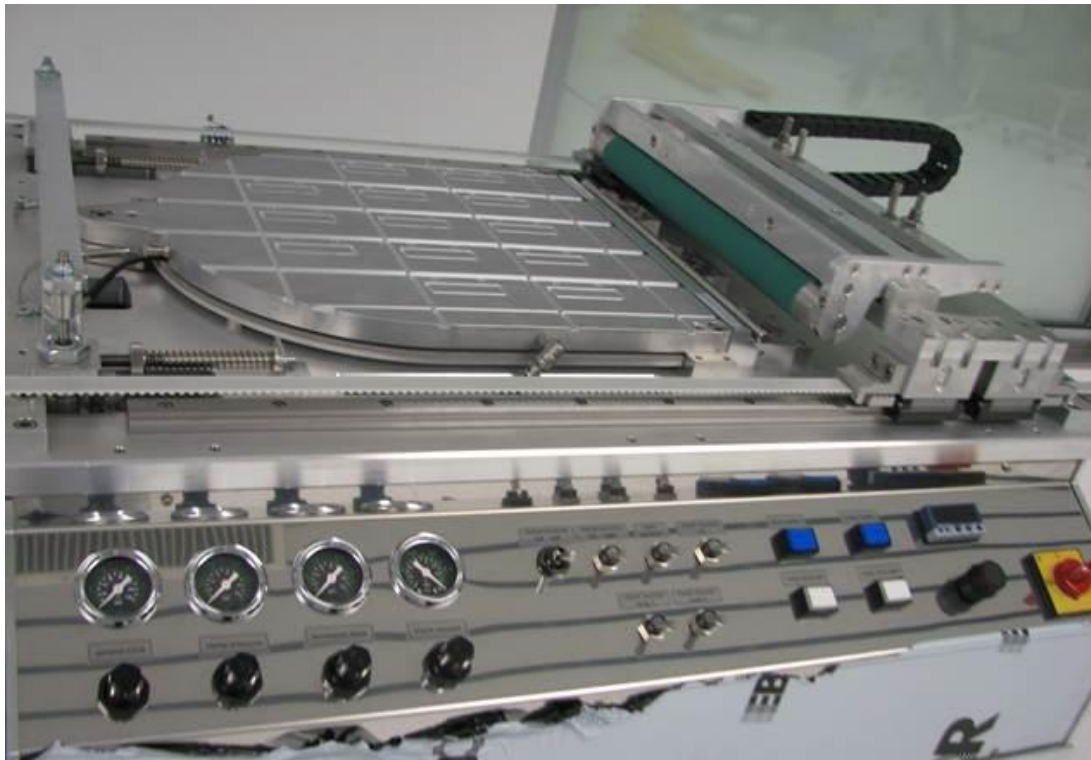
Figure II.3. The rolling laminator machine used in the solvent bonding method, designed by EVG® for the Lab On Foil Integrated Project.
