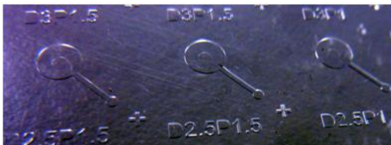
Figure 3.5. PDMS master mould with different valve designs for hot embossing.
