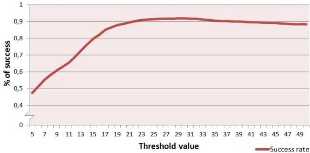
Fig. 13 - Descriptor classification accuracy depending on threshold
