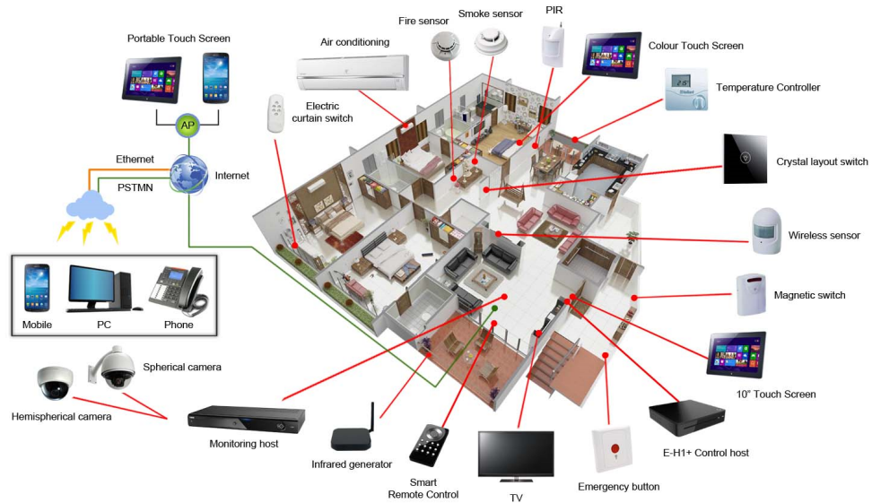
Figure 1.1: Image of an AmI environment with sensors, actuators, processing units and communication systems
