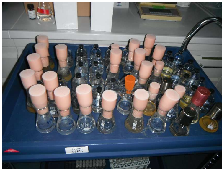
Figure 5.2. Conical flasks (aerobic) and serum bottles (anaerobic) utilized during the nitrifying experiment. The yellowish coloration of some of the macrocosms is caused by ferric iron precipitates formed in the monimolimnetic samples when exposed to air.
