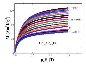
Figure 2. Magnetic field dependence of the isothermal magnetization for Gd<sub>1.7</sub>Ce<sub>0.3</sub>Fe<sub>1.7</sub>.
