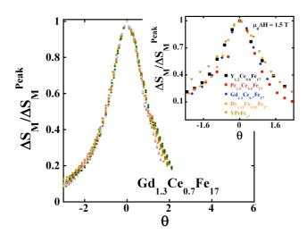
Figure 4. Master curve for  $Gd_{1.3}Ce_{0.7}Fe_{17}$  obtained using two temperatures of reference (see text for details). The inset shows a comparison of the master curves for the studied pseudo-binary alloys under a magnetic field change  $\mu_0\Delta H = 1.5$  T.
