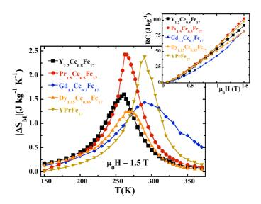
Figure 3. Temperature dependence of the magnetic entropy change for  $R_x R'_{2-x} Fe_{17}$  alloys under  $\mu_0 \Delta H$  = 1.5 T. Inset shows the field dependence of refrigerant capacity.
