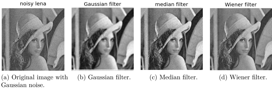
Figure 2.7: Result of applying different denoising techniques to an image corrupted with Gaussian noise.
