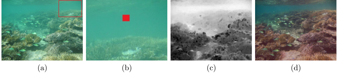
Figure 3.1: Waterlight detection from Red channel. (a) Original image, the red rectangle marks the region from where waterlight was extracted (b) In red, exact pixel location of waterlight within the rectangle marked in (a) (c) Red Channel of the original image (d) Final restoration result.
