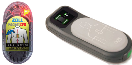
Figure 1.10: CPR quality feedback devices based on accelerometers: PocketCPR (Zoll) and CPRmeter (Laerdal), from left to right.
