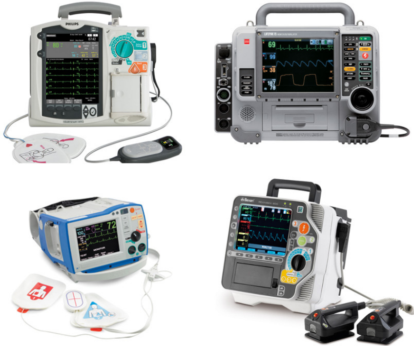
Figure 1.4: Monitor/defibrillators from different commercial brands. From left to right and from top to bottom: Heartstart MRx (Philips), Lifepak 15 (PhysioControl), R Series ALS (Zoll), Reanibex 800 (Bexen cardio).
