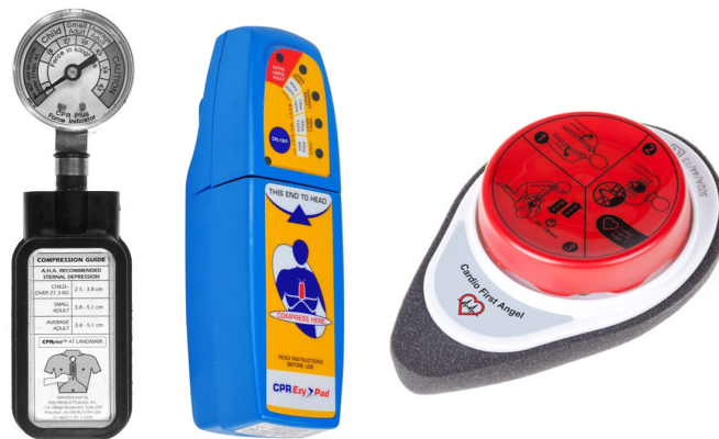
Figure 2.7: CPR quality feedback devices based on force or pressure sensors: CPRplus (Kelly Medical Products), CPREzy (Health Affairs) and Cardio First Angel (Schiller).
