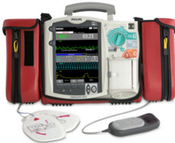
Figure 2.15: Heartstart MRx with Q-CPR for CPR feedback.
