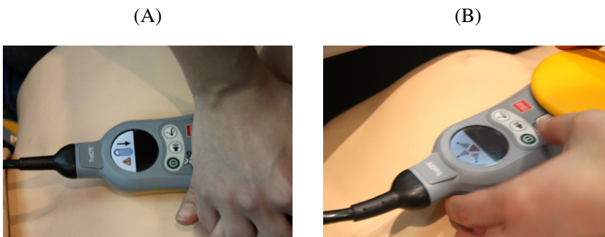
Figure 5.10: Alerts displayed by TrueCPR during the long-distance train measurements. (A) shows an alert indicating that the distance between the back pad and the chest pad is incorrect, and that the back pad should be repositioned. (B) indicates that electronic noise is interfering with the device.
