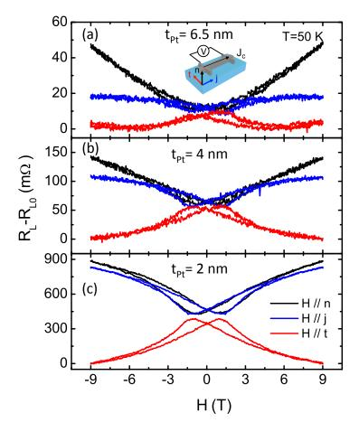
Figure 7.5: Longitudinal resistance  $R_L$  for (a) (001)IN(7), (b) (001)IN(4) and (c) (001)IN(7) as a function of the applied magnetic field, H, along  $\hat{t}$  (red curves),  $\hat{j}$  (blue curves) and  $\hat{n}$  (black curves).  $R_{L0}$  is the subtracted background. The orientations of the applied magnetic field and the measurement configuration are sketched in the inset. All measurements are done at 50 K.
