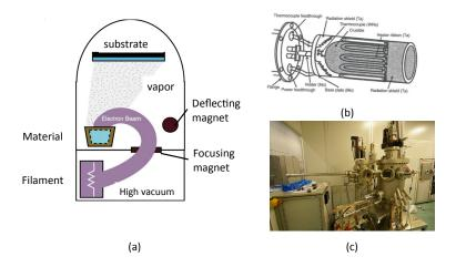
Figure 3.5: (a) Schematic representation of an e-beam evaporation process. (b) Schematic representation of an effusion cell. (c) UHV evaporator by *Createc* used in this work.
