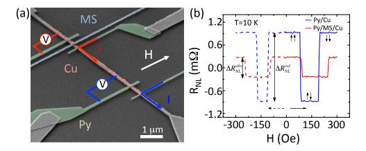
Figure 5.1: (a) Colored SEM image of two Py/Cu LSVs, one of them with a MS wire in between the Py electrodes. The measurement configuration, the direction of the applied magnetic field (H) and the different materials (Py, MS and Cu) are shown. (b) Non-local resistance as a function of H at 10 K for a Py/Cu LSV without (blue line) and with (red line) the MS wire in between the electrodes. The solid (dashed) line represents the increasing (decreasing) sweep of H.
