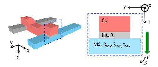
Figure 5.5: Schematic representation of a device and its transverse cut where the Cu channel, an interfacial layer and the MS wire are presented. The interfacial layer is inserted to take into account the spin memory loss.
