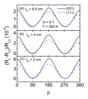
Figure 7.2: Angle-dependent longitudinal magnetoresistance measurements at 9 T and 300 K when rotating the magnetic field in a plane perpendicular to the current (i.e., as a function of  $\beta$ ) for epitaxial (001) and (111) Pt/CFO samples grown in situ with (a) 6.5 nm, (b) 4 nm and (c) 2 nm of Pt.  $R_L$  is the measured resistance and  $R_{L0}$  is the subtracted background.
