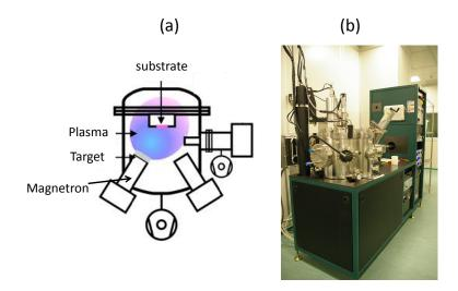
Figure 3.4: (a) Schematic representation of the magnetron sputtering process. (b) UHV 7-gun sputtering system by AJA used in this work.
