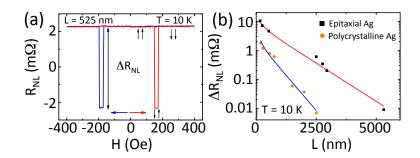
Figure 4.3: (a) Non-local resistance as a function of the applied magnetic field at 10 K for a Py/Ag LSV with epitaxial Ag where L=525 nm. The spin signal is tagged as  $\Delta R_{NL}$ . (b) Spin signal as a function of the distance L between the electrodes at 10 K in Py/Ag LSVs. The solid black (orange) squares (circles) are the experimental data for the epitaxial (polyscrytalline) Ag and the red (blue) line is the fit to Eq. 2.14.
