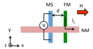
Figure 2.7: Schematic representation of a spin Hall device with only one FM electrode. The geometrical parameters, direction of the applied magnetic field and the measurement configuration to detect the ISHE are shown.
