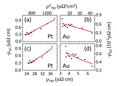
Figure 5.6: (a) Spin Hall resistivity as a function of the square of the total resistivity (a) for Pt and (b) for Au (black dots). The red solide line is a fit of the data to Eq.5.6, where the phonon skew scattering contribution is neglected. Spin Hall resistivity as a function of the total resistivity for (c) Pt and (d) Au (black dots). The red solid line is a fit of the data to Eq. 5.8, taking into account phonon skew scattering contribution.
