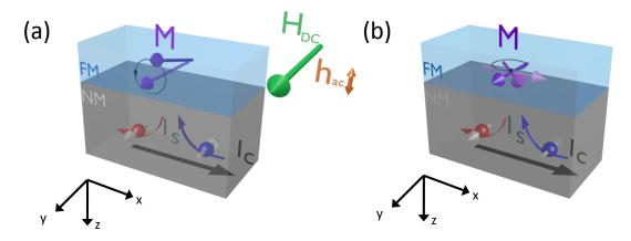
Figure 1.5: (a) Spin-pumping technique. In this case, ferromagnetic resonance induced by an *ac* field in the FM injects a *dc* spin current into the NM, which is converted into charge current due to ISHE. (b) Spin-transfer torque technique. This is the reciprocal technique, where a charge current through the NM will create a spin current due to SHE, that will induce the precession of the magnetization of the adjacent FM.
