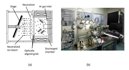
Figure 3.6: (a) Schematic representation of an Ar-ion milling process. (b) Ar-ion miller equipment by 4-WAVE used in this work.
