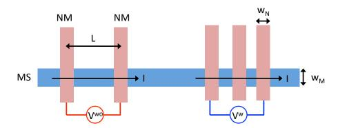
Figure 2.8: Schematic representation of the two necessary devices to estimate the shunting coefficient. The device in the left is the reference, whereas the one in the right, with the middle NM wire in between the voltage probes, measures the voltage drop due to the additional wire. Both devices have the same dimensions, where L is the separation between the voltage probes and  $w_N$  and  $w_M$  are the widths of the NM metal and MS, respectively. Note that all the NM are of the same width.
