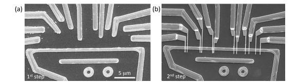
Figure A.1: (a) First step of the fabrication process where the NM channel is defined. (b) Second step of the fabrication process, where the FM electrodes are deposited on top of the NM channel.
