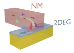
Figure 2.9: Schematic representation of the detection of the IREE, where a 3D spin current  $(I_s)$  is injected from a NM channel into a 2D electron gas (2DEG), creating a 2D charge current  $(I_c)$ .
