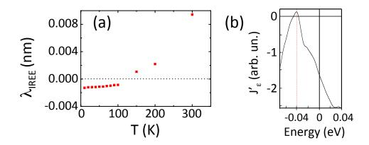
Figure 6.3: (a) Temperature evolution of the IREE length of Bi as obtained from a SA device. (b) Energy dependence of the spectral current density  $j_E'(E)$  calculated by using  $s_\lambda(k_{\parallel})$  for  $n_\lambda(k_{\parallel})$ .
