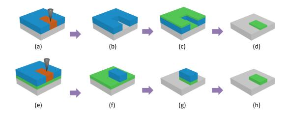
Figure 3.1: The main steps involved in the fabrication process using positive resist (a-d) or negative resist (e-h). (a) Exposure of the pattern on top of a positive resist. (b) Developing of the exposed part. (c) Material deposition. (d) Lift-off of the resist. (e) Exposure of the pattern on top of negative resist. (f) Developing process. Only the exposed part remains after this step. (g) Etching of the material that is not protected by the resist. (f) Lift-off to remove the resist.
