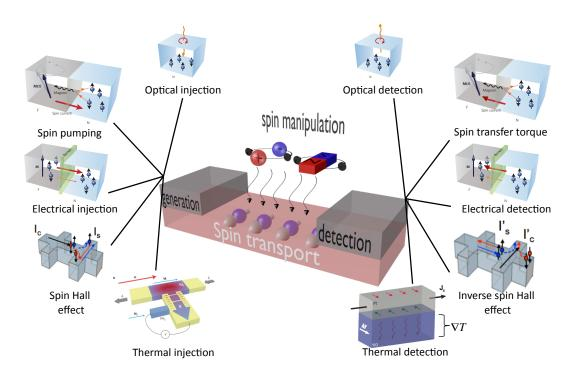
Figure 1.1: Sketch with key ingredients for the performance of a spintronic device: (i) Generation and detection of pure spin currents by different methods; (ii) Spin transport; (iii) manipulation of the transported spin information by electric or magnetic fields. Fig. adapted from Refs. [17], [37] and [43].
