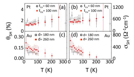
Figure 5.4: Spin Hall angle (a) and spin Hall conductivity (b) of Pt as a function of temperature obtained from two devices with  $t_{Pt}$ = 15 nm and different  $t_{Cu}$  (see legend). Spin Hall angle (c) and spin Hall conductivity (d) of Au as a function of temperature obtained from two devices with  $t_{Au}$  = 80 nm and different d (see legend).
