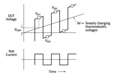
Figure 3.8: Schematic representation of the DC reversal technique. Figure taken from Ref. [5].
