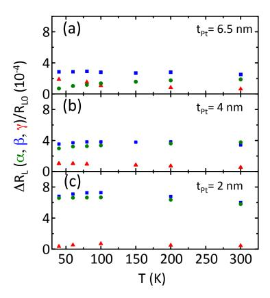
Figure 7.4: The amplitude of the ADMR at 9T as a function of temperature for the three different angles:  $\alpha$  (green circles),  $\beta$  (blue squares) and  $\gamma$  (red triangles) for (a) (001)IN(7), (b) (001)IN(4) and (c) (001)IN(2) samples.
