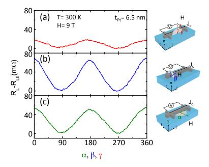
Figure 7.3: Angle-dependent longitudinal magnetoresistance measurements at 9 T and 300 K for the (001)IN(7) sample along (a)  $\gamma$ , (b)  $\beta$  and (c)  $\alpha$  rotation planes.  $R_L$  is the measured longitudinal resistance and  $R_{L0}$  the subtracted background. The sketches in the right define the Hall bar geometry, the longitudinal measurement set-up and the angles  $\alpha$ ,  $\beta$  and  $\gamma$ .
