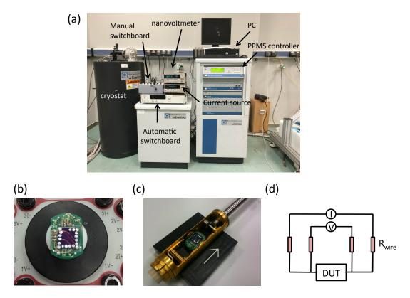
Figure 3.7: (a) PPMS equipment by *Quantum Design* and the measurement instruments (automatic and manual switchboards, nanovoltmeter and current source) used in this thesis. (b) A device glued in a puck and contacted to it by copper wires and indium. (c) Sample rotator with a device ready to be introduced into the cryostat. (c) Four-point measurement configuration.
