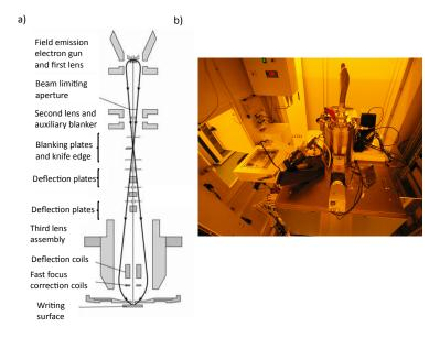
Figure 3.3: (a) Schematic representation of the SEM column in the eBL. (b) Raith 150-TWO equipment used in this work.
