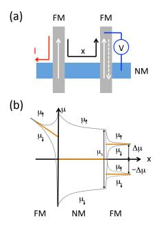
Figure 2.2: (a) Schematic representation of a LSV, where the FM injector, NM channel and the FM detector are shown, together with the non-local measurement scheme. (b) Evolution of the electrochemical potential (orange line) along  $\hat{x}$  direction. Electrochemical potential of spin-up and spin-down electrons (grey line). The solid (dashed) line represents the electrochemical potential when both FM have a parallel (antiparallel) magnetization. Figure adapted from Ref. [6].
