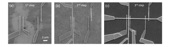
Figure B.1: (a) First step of the fabrication process where the FM electrodes are defined. (b) Second step of the fabrication process, where the MS is inserted in the middle of one of the pairs of the FM electrodes. (c) Third step where the NM channel is patterned, bridging the FM electrodes and the middle MS wire.
