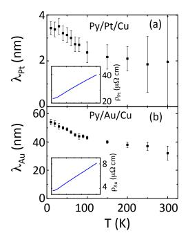
Figure 5.2: Spin diffusion length of (a) Pt and (b) Au as a function of temperature obtained from spin absorption experiments. Insets: (a) Pt and (b) Au resistivity as a function of temperature. Note that the temperature scale in the inset is the same as the one in the main figure.
