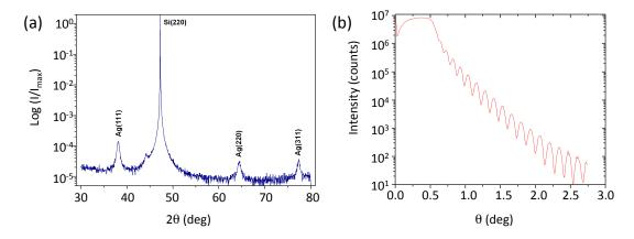
Figure 3.10: (a) X-ray diffraction measurement of a 40-nm-thick polycrystalline Ag thin film on top of a <110> Si substrate. (b) Intensity profile for the reflectivity measurement of a 30-nm-thick Au thin film.
