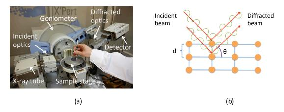
Figure 3.9: (a) The X-ray diffractometer used in this work with the different parts labeled. (b) Schematic representation of how X-rays scatter with a crystalline structure.
