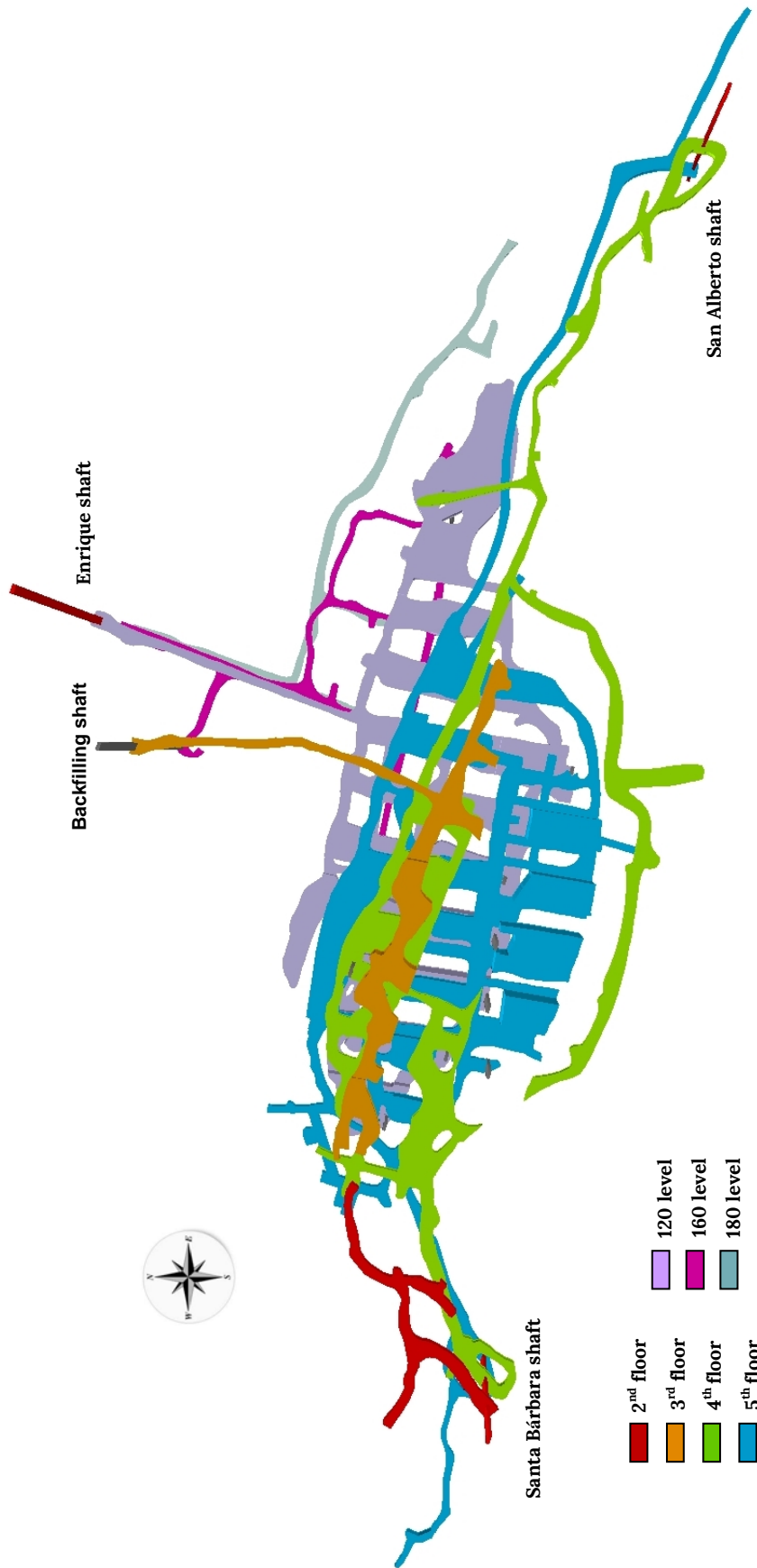
Figure. 2.18. Cueva de la Mora exploitation (1971). Plan of the 2 nd , 3 rd , 4 th , 5 th floors, and 120, 160 and 180 levels.
