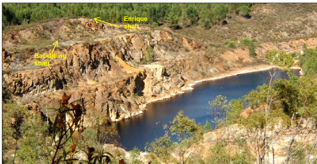
Figure 2.4. View of the northern slope formed by three benches of 10 m high, photograph taken from cerro Castillejito.
