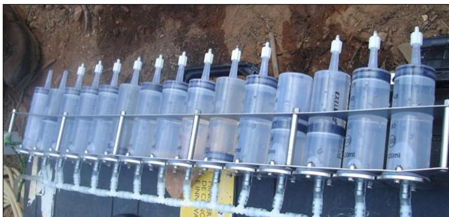
Figure 5.1. Syringe-sampling system constructed for the detailed sampling of the chemocline.
