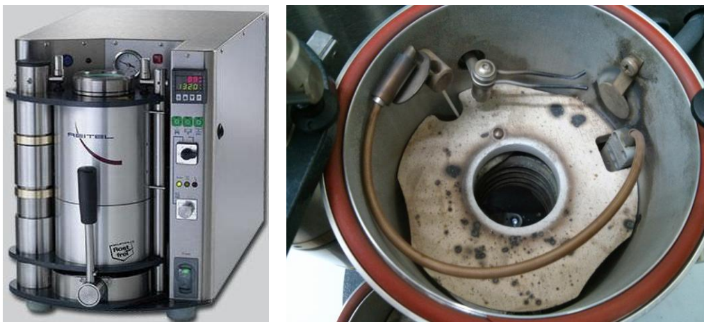
Figure 2.1. Picture of the used Reitel Indirect Compact induction furnace (left). View of the coil and thermocouple of the furnace (right).
