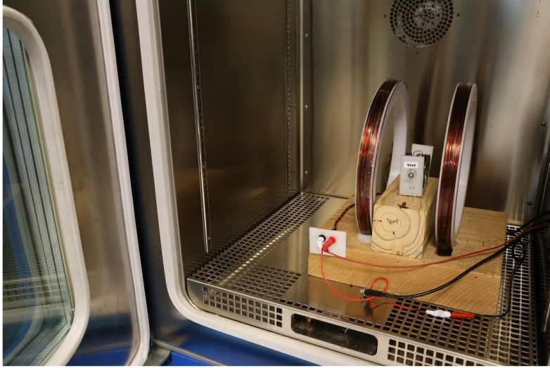
Figure 5.6. Set-up for the ME characterization under temperature.
