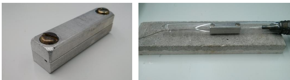
Figure 2.4. Picture of aluminium pieces used for the annealing of the ribbons (left). Picture of the whole system used for the annealing process (right).
