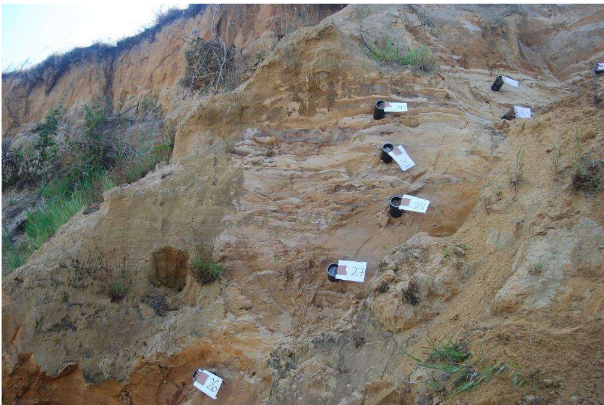
Figure 3.10. Beds 15 to 21 (Poyambre 26 to 33), composed of yellow and beige sands alternating with thin clay layers.
