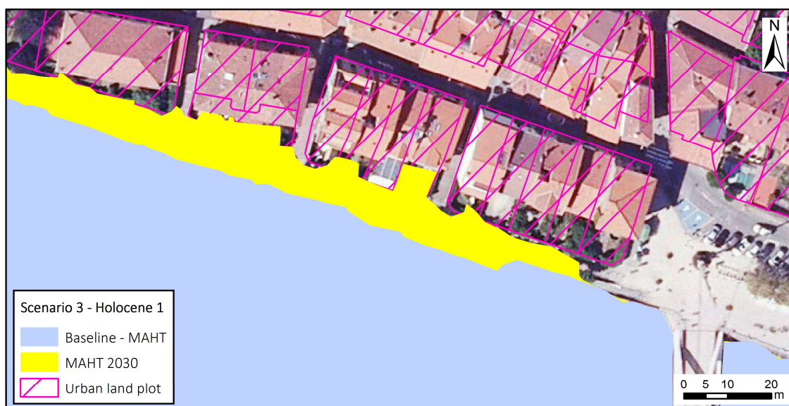
Figure 5.7. Estimation of affected assets by overlapping flood maps on urban land plots.
