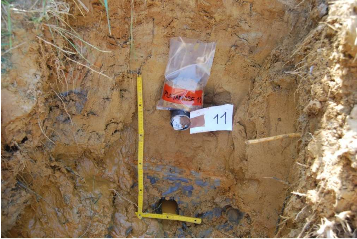
Figure 2.12. Sample 11: steel tube inserted into the sediment and sub-sample bag.
