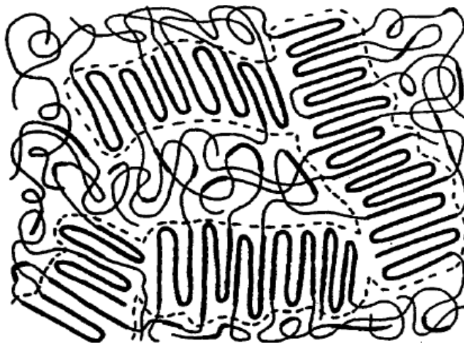
Figure II. Model of microstructure of chain conformation in the COPs materials with large amorphous, rubbery regions between crystalline or rigid domains.
