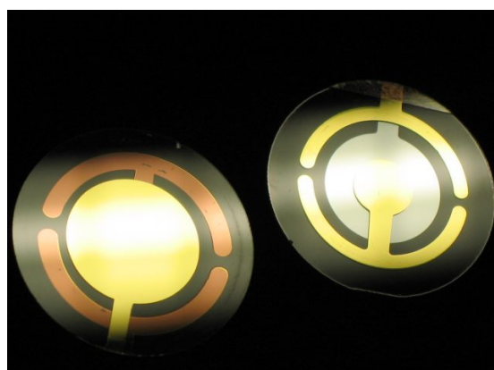
Figure II.16. Sensor of the Quarz Crystal Microbalance with Dissipation(QCM-D).
