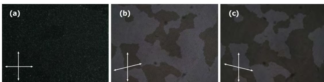
Fig. 48: Textures of a dark conglomerate phase: (a) between crossed polarizers; (b) and (c) chirality domains as seen uncrossing the polarizers in both senses due to opposite optical activity.
