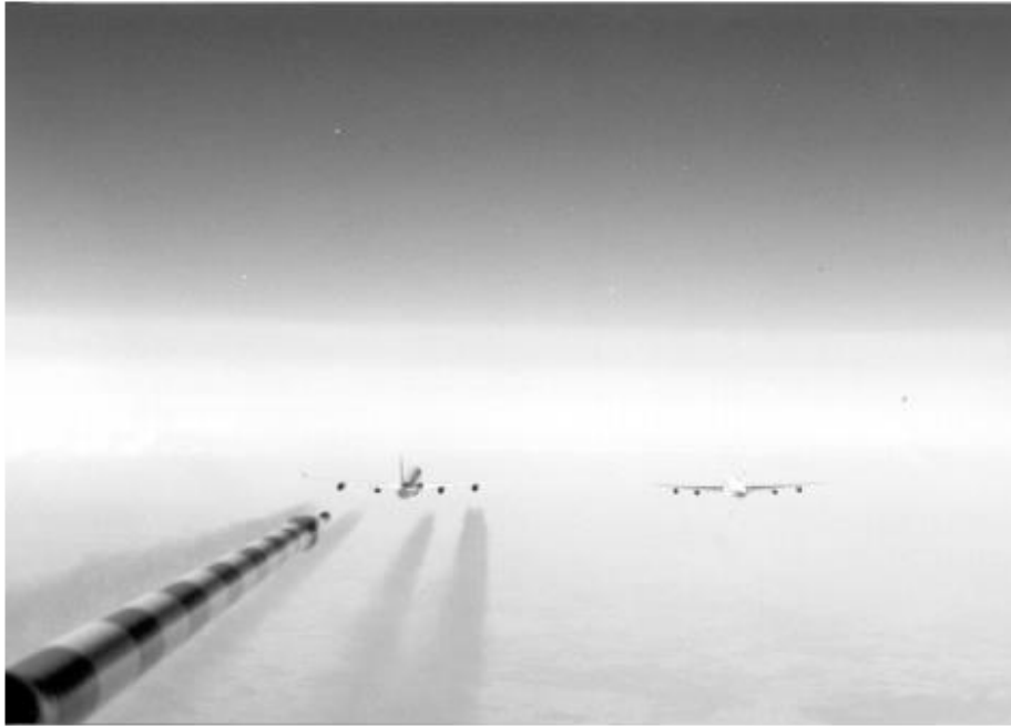
Figure 2-4: Airbus A340 producing contrails and Boeing B707 without contrails flying at 10.5 km altitude (Schumann 2000)
