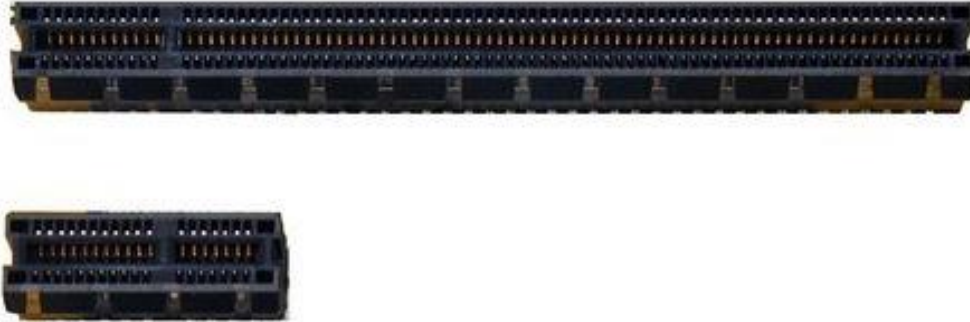
Figure 2-9. PCI Express x16 (top, 164 pins) and PCI Express x1 (bottom, 36 pins) connectors (image taken from [29])
