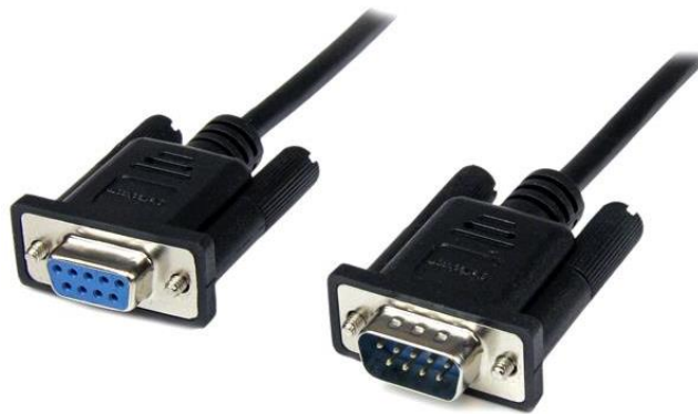
Figure 2-10. DB9 female (left) and male (right) for RS-232 communications (image taken from [32])
