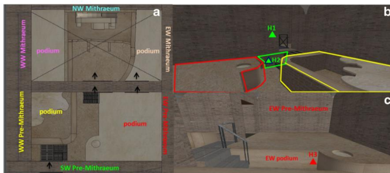
Fig. 6 Positioning sensors. a pre-Mithraeum and Mithraeum plan; b , c sensor placement in the pre-Mithraeum: H1 and H2 ( b ); H3 ( c )
