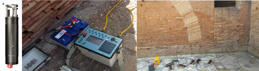
Figure 10. a) Sound water velocity (MONITOR SVP - Valeport); b) Georesistivimeter (IRIS Syscal Pro); c) Seismograph (Geometrics Geode, yellow box + piezoelectric accelerometers, black electrodes).
