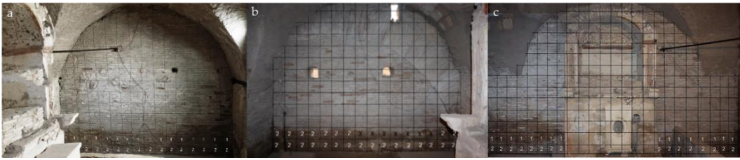
Figure 28. Modular grid installation in Mithraeum room, with the Stage method values assignment. a) East wall; b) west wall; c) north wall.
