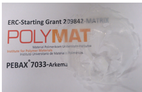
Figure 3. 5 Samples of cast membranes obtained with different Pebax®XX33 grades. a) Pebax®2533, b) Pebax®5533 and c) Pebax®7033
