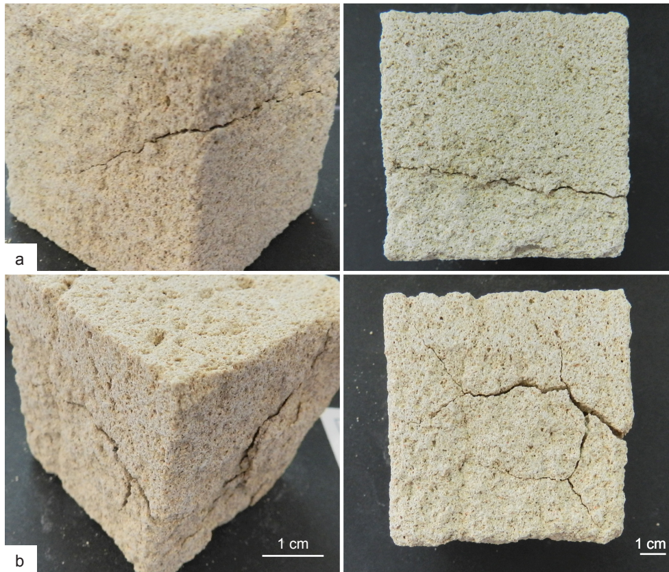
Figure 87. Detailed images of the broken Bateig stone specimens after the sodium sulfate aging test. a) Blank specimen; b) Sample treated with \text{Ca}(\text{OH})_2 nanoparticle at 25 g/l concentration exposed to the yeast system environment.
