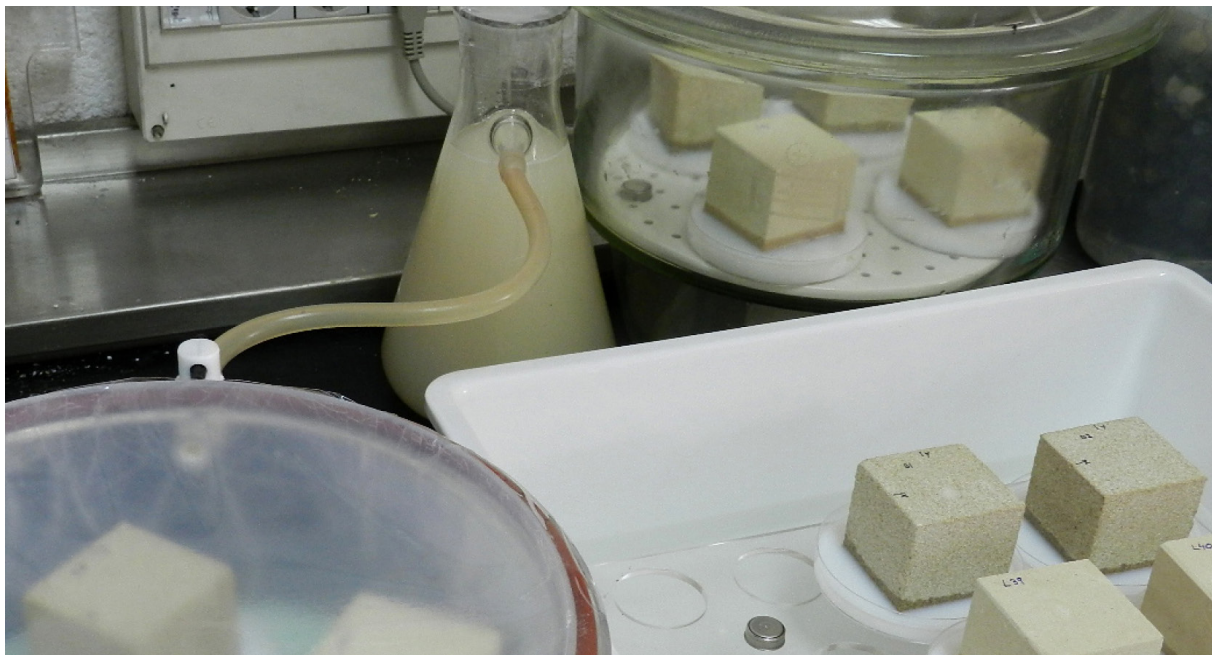
Figure 40. Setup of the experiment at the laboratory showing the limestone specimens and the consolidating product based on Ca(OH) 2 nanoparticles, in the three environmental conditions. To the left, stone specimens (5 cm 3 ) connected to the flask with the yeast fermentation; in the back, specimens inside the closed container at high humidity; to the right and front, stone specimens exposed to the ventilate laboratory conditions.
