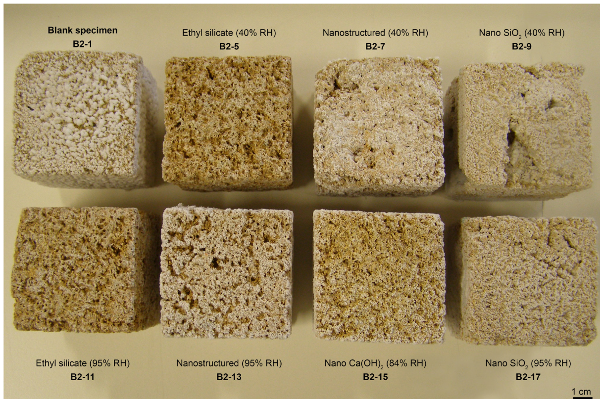
Figure 88. Calcarenite stone cubic specimens after treatment with different consolidation products exposed to different relative humidities (RH) (dry (40% RH) and very humid (84-95% RH) environments) after marine aerosol aging test and before being cleaned with water following the standard UNE-EN 14147 (2004).
