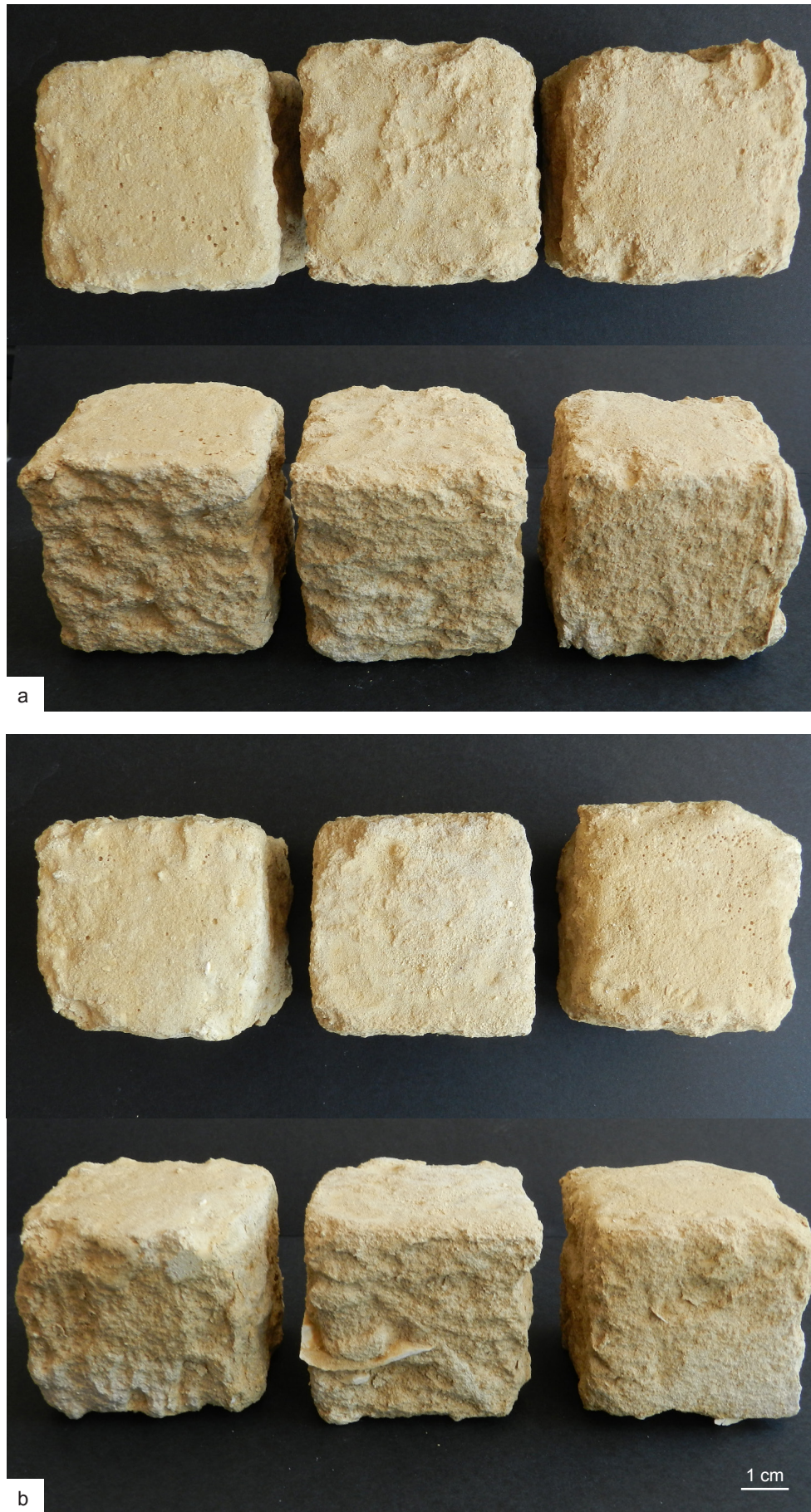
Figure 85. Front and side views of Lecce stone treated samples after the sodium sulfate salt crystallization aging test and prior to desalination immersion baths. a) Samples treated with the \text{Ca(OH)}_2 nanoparticles at 5 g/l concentration. From left to right: L34 (laboratory conditions), L36 (closed container) and L38 (yeast system); b) Samples treated with the \text{Ca(OH)}_2 nanoparticles at 25 g/l concentration. From left to right: L40 (laboratory conditions), L42 (closed container) and L44 (yeast system).
