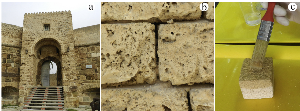
Fig. 1. Provenance, weathering and consolidation of stone specimens: a: façade of the Spanish fortress of Bizerte; b: alveolar weathering in decayed stones; c: brush application of the consolidating treatment in stone cubic specimens.
