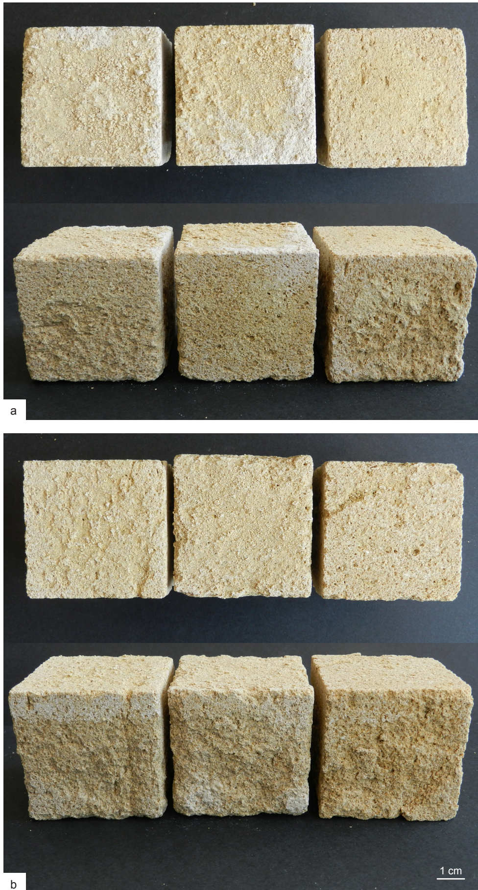
Figure 86. Front and side views of Bateig stone treated samples after the sodium sulfate crystallization aging test and prior to desalination immersion baths. a) Samples treated with the \text{Ca(OH)}_2 nanoparticles at 5 g/l concentration. From left to right: B50 (laboratory conditions), B52 (closed container) and B54 (yeast system); b) Samples treated with the \text{Ca(OH)}_2 nanoparticles at 25 g/l concentration. From left to right: B2 (laboratory conditions), B4 (closed container) and B6 (yeast system). The blank specimen pictures of Bateig stone are shown in Fig. 87.
