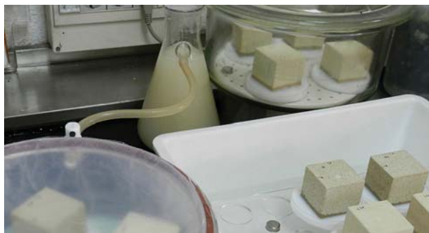
Fig. 1 Setup of the experiment at the laboratory showing the limestone specimens and the consolidating product based on \text{Ca}(\text{OH})_2 nanoparticles, in the three environmental conditions. To the left, stone specimens ( 5 \text{ cm}^3 ) connected to the flask with the yeast fermentation; in the back, specimens inside the closed container at high humidity; to the right and front, stone specimens exposed to the ventilate laboratory conditions
