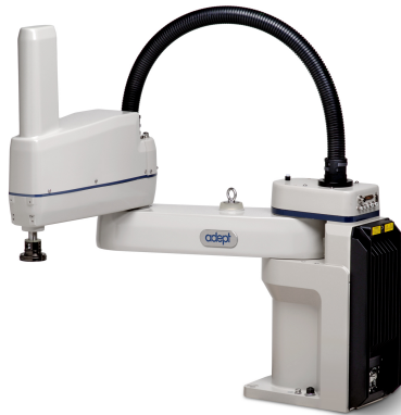
Figure 1.2. Picture of the Scara robot Cobra-800 by Adept [2].
