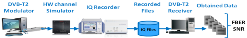
Figure 23. Laboratory measurements set-up
