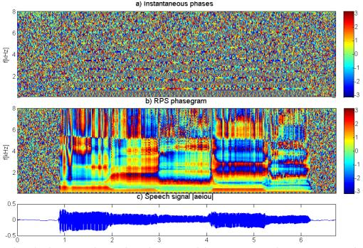
Figure 2: Phasegrams of a voiced speech segment with five continuous vowels. (a) Instantaneous phases. (b)Relative phase shift (c) Signal waveform.
