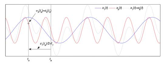
Figure 1: Graphical interpretation of the RPS transformation: for an analysis instant  $t_a$  the RPS of k is the phase shift of that component with respect to the fundamental component at the point where the period of the fundamental component starts ( $t_o$ ).
