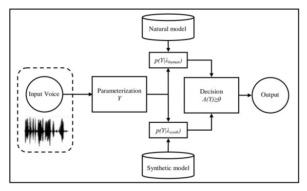
Figure 4: SSD system structure.
