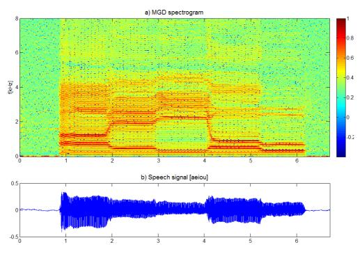
Figure 3: MGD spectrogram of a voiced speech segment with five continuous vowels.
