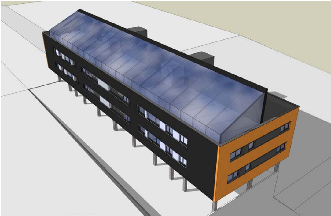
Fig. 2. Infografía del invernadero situado en la cubierta del edificio. Infographic of the greenhouse located on the roof of the building.
