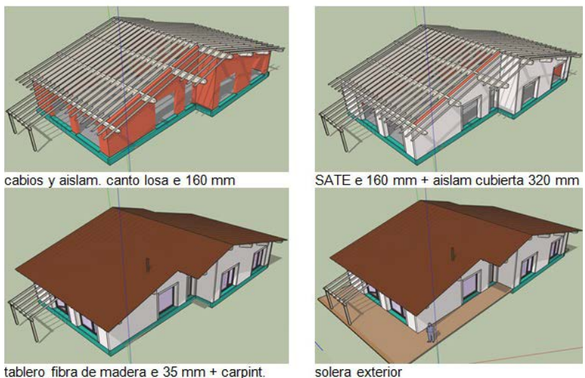
Fig. 5. fases constructivas 5 a 8. Construction phases 5 to 8.
