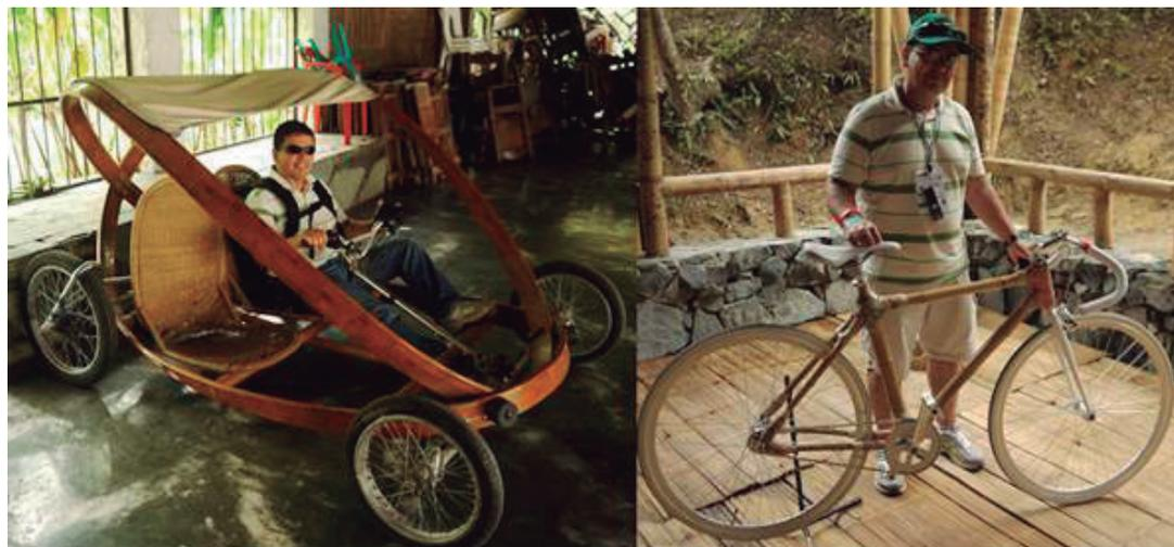
**Fig 5.** Prototipo de coche realizado en bambú laminado y bici hecha con caña natural. Vehicle prototype made on laminated bamboo and bike made on natural cane
