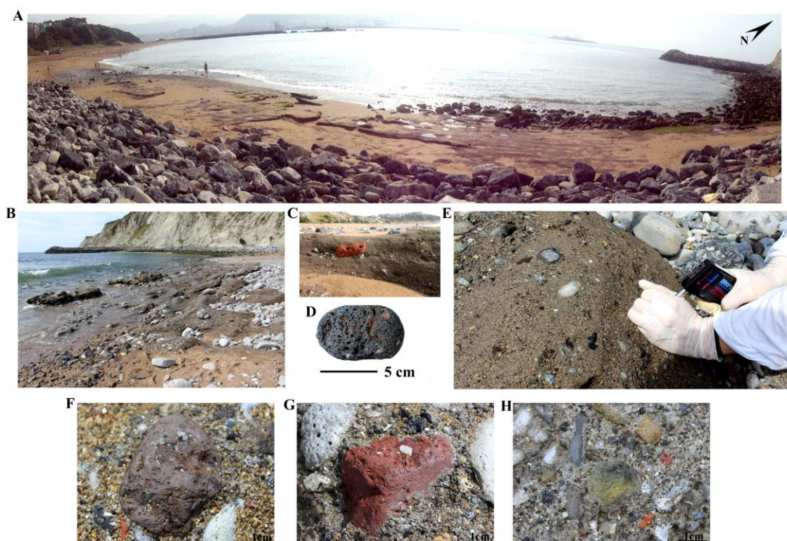
Figure 3.2. A) Overview of the indurated and isolated residual platform and benches. B) Example of the area examined with in situ Raman spectroscopy in the northernmost part of the beach. C) Detail of a brick trapped in the beachrock. D) Exemplar of a typical slag found in the beach. E) In situ Raman spectroscopy analysis being carried out in the beachrock. F-H) Wastes that can be found cemented in Arrigunaga beach.
