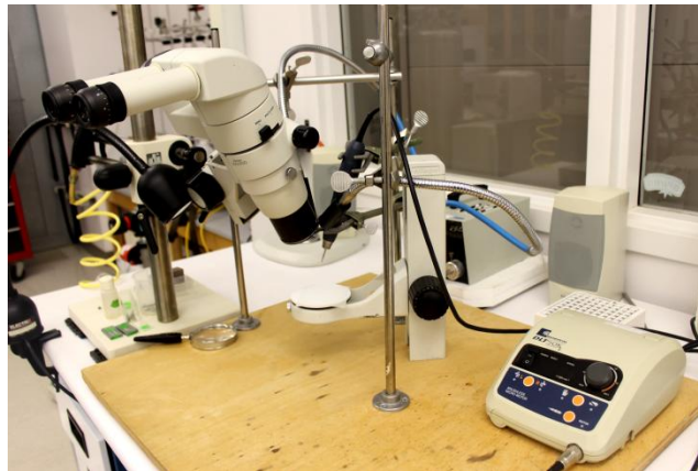
Figure 3.16. Image of the microscope-mounted drill assembly used for the collection of cement samples.
