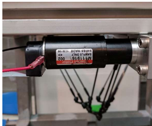
Figure 44: Motor and gearhead mounted on a previous prototype.
