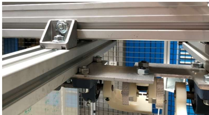
Figure 59: Mounting of the prototype to the structure.
