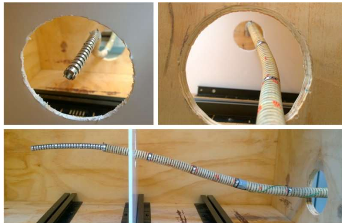
Figure 1: Example of a continuum robot for on-wing inspection/repair of gas turbine engines (3)
