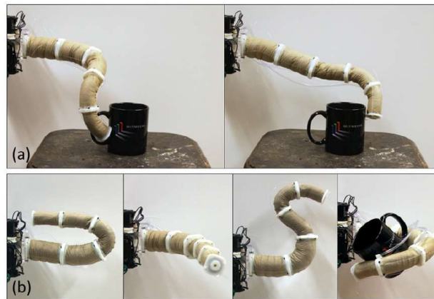
Figure 22: Different positions for the manipulator made of ground coffee.
