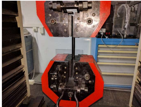
Figure 9: Traction test on 10-mm nylon bars.
