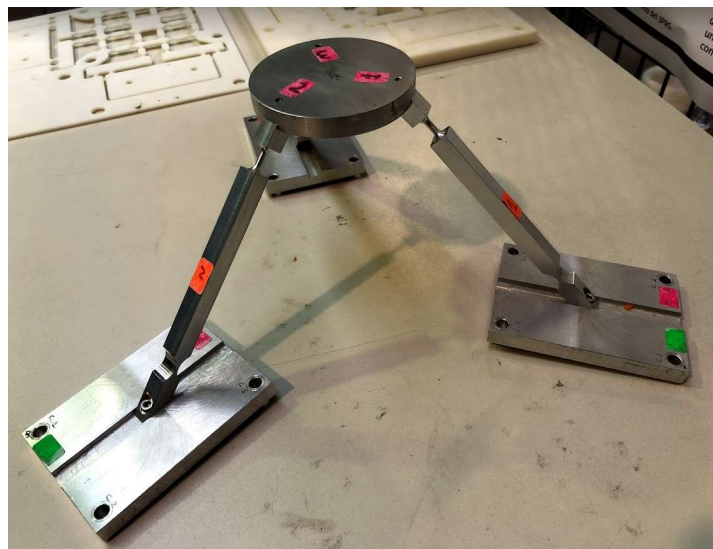
Figure 2: Example of Compliant Mechanism Using Flexure Hinges (4)
