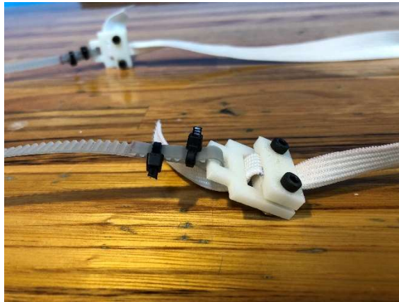
Figure 49: Detail of how the clamps work.
