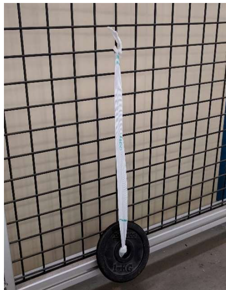
Figure 46: Testing for permanent deformations on the rubber band.
