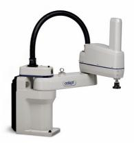
Figure 1.4: SCARA robot. Courtesy of Adept
