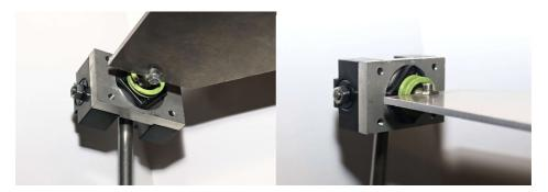
Figure 14.9: Universal joint seen from different views
