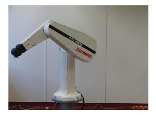
Figure 1.3: PUMA robot. Courtesy of Unimation
