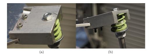
Figure 14.13: Spherical joint: (a) union with the platform; (b) spring
