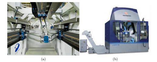
Figure 1.21: Two machine centres with PKMs: (a) Cosmo Center PM-600. Courtesy of Okuma; (b) Vertical Turning Machine V100. Courtesy of Index
