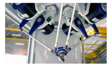
Figure 1.20: Hexa 6-DOF parallel manipulator
