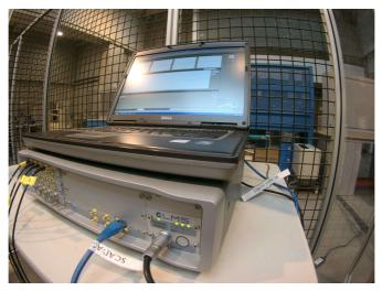
Figure 15.29: Siemenes LMS TestLab analyser
