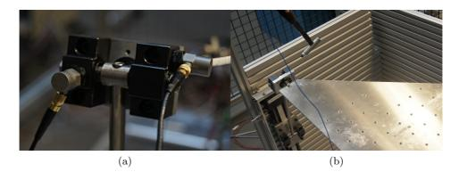
Figure 15.32: Measurement along Y-axis: (a) accelerometer on joint U in X- and Y-axes direction; (b) impulse in Y-axis direction
