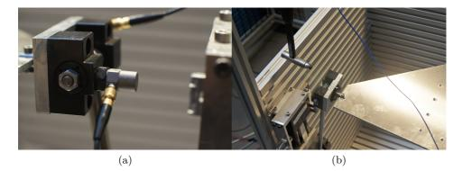
Figure 15.31: Measurement along X-axis: (a) accelerometer on joint U in X-axis direction; (b) impulse in X-axis direction
