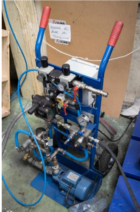
Figure 2.4. Portable pump of the test bench
