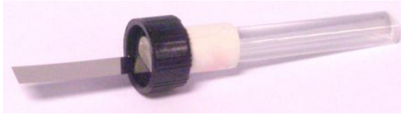
Figure 25. Magnetoelastic ribbon clamped on one end to a glass tube, enclosed in a plastic tap of the lubricant oil recipient.
