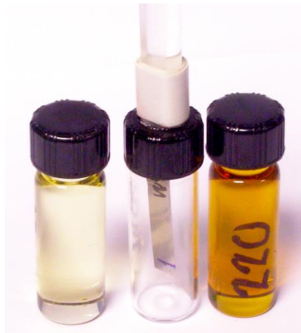
Figure 26. The sensing element, attached to the cap of the vial, is completely immersed in the oil under test.
