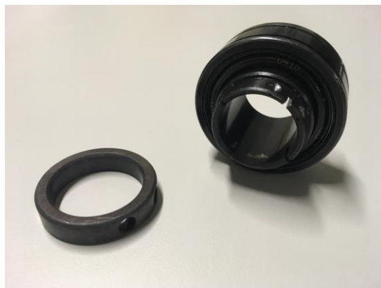
Figure 26. Image of the bearing installed in the test bench.
