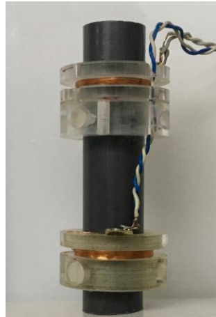
Figure 30. Pick-up (top) and compensation coil (bottom) in the sensor prototype.
