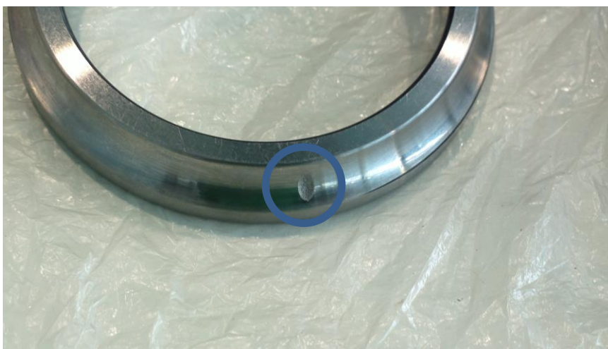
Figure 33. Detail of the inner race fault.
