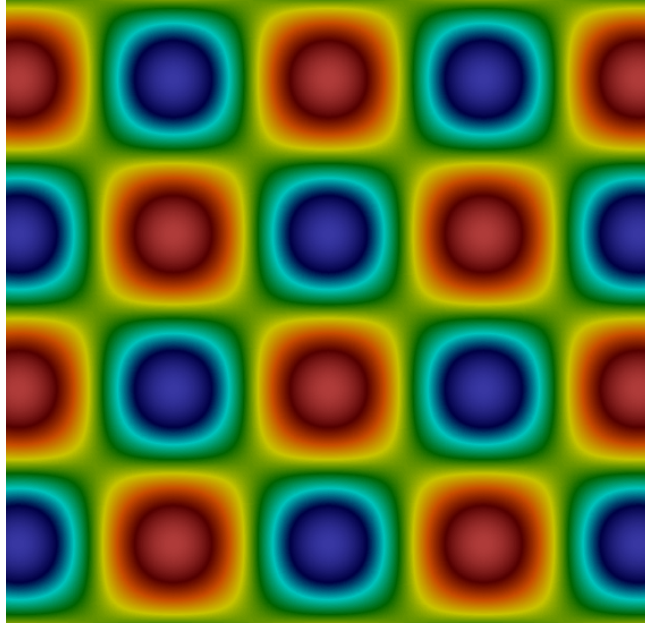
FIGURE 4.4: Taylor-Green test case x-component velocity field representation
