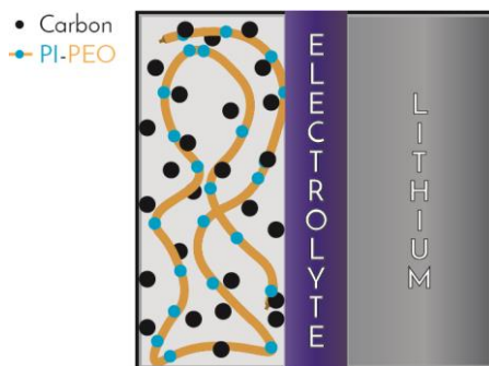
Figure 3.8. Schematic diagram of a lithium cell composed of polyimide-polyether copolymers and carbon as cathode.
