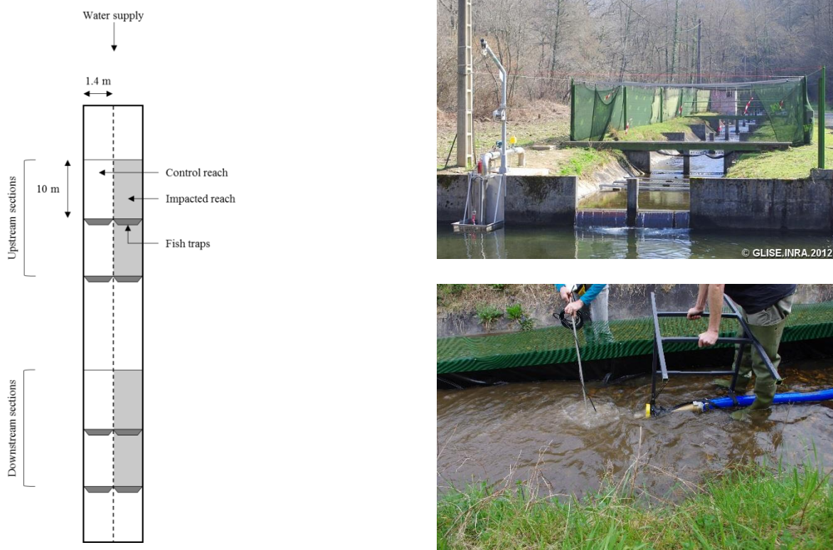
Figure 4.1 Experimental design set up in the semi-natural channel of the Lapitxuri. Eight reaches were used. Four reaches were impacted by the flood (left bank – in grey) and four reaches served as controls (right bank – in white).
