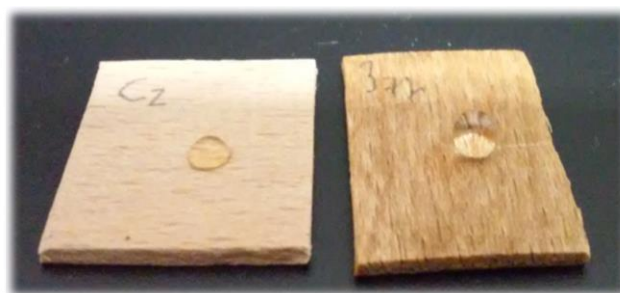
Figure 5.10. Difference on water wettability between beech veneer before and after 72h of immersion.
