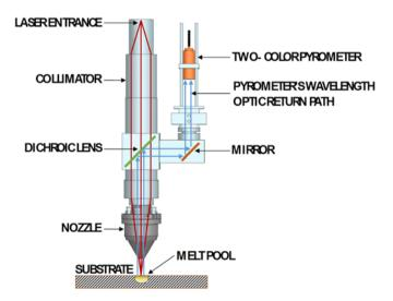
Fig. 3. Optical paths of the laser beam and the two-color pyrometer.
