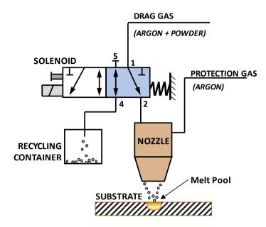
Fig. 5. Scheme of the powder flux regulation system, where the solenoid is in position 1.
