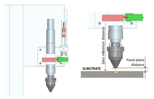
Fig. 7. Scheme of the clad height measuring system.
