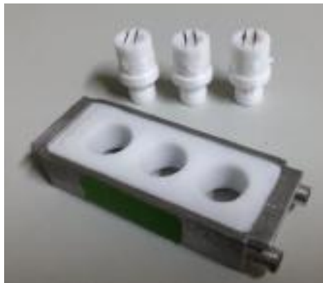
Figure 2.4. Homemade chamber and PTFE circular wells for the formation of GUVs attached to a platinum wire.
