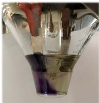
Figure 3.2 a) Electrochemical cell setup. b) Cyclic voltammograms of the electrochemical polymerization of ProDOT-COOH (10 -2 M) in 0.1 M \text{TBAClO}_4 acetonitrile solution, using a 1 cm 2 platinum working electrode, switching potential from -0.05 V to 1.7 V at a 20 mV s -1 scan rate
