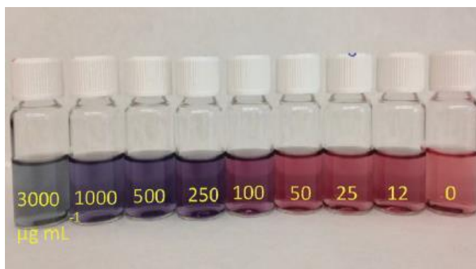
Figure 1.10: Photographs of the sensing system based on pyridine-gold-zein interactions involving pyridine-functionalized single-chain nanoparticles in the presences of decreasing concentrations of zein.
