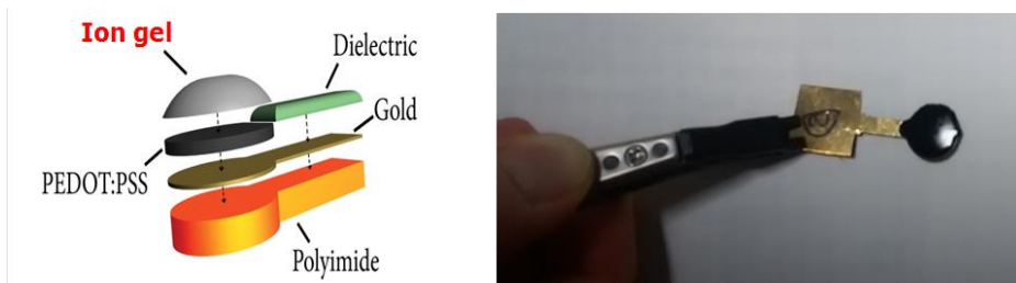
Figure 46. An exploded view of the electrode and all of the different materials used (left). A photograph of the electrode with the ion gel deposited on top (right).
