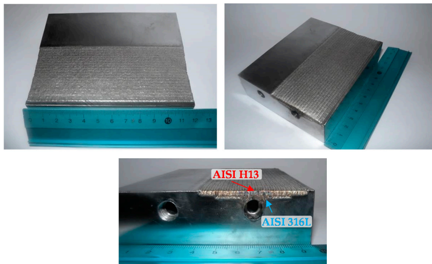
Figure 4. Final part after finishing the LMD process.
