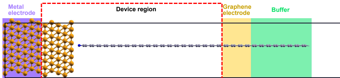
Figure 4.7: Setup for transport calculations of metal-graphene edge contacts with metal electrode (blueish) and graphene electrode (yellow) attached to the device region. The black frame indicates the unit cell used in the calculations.
