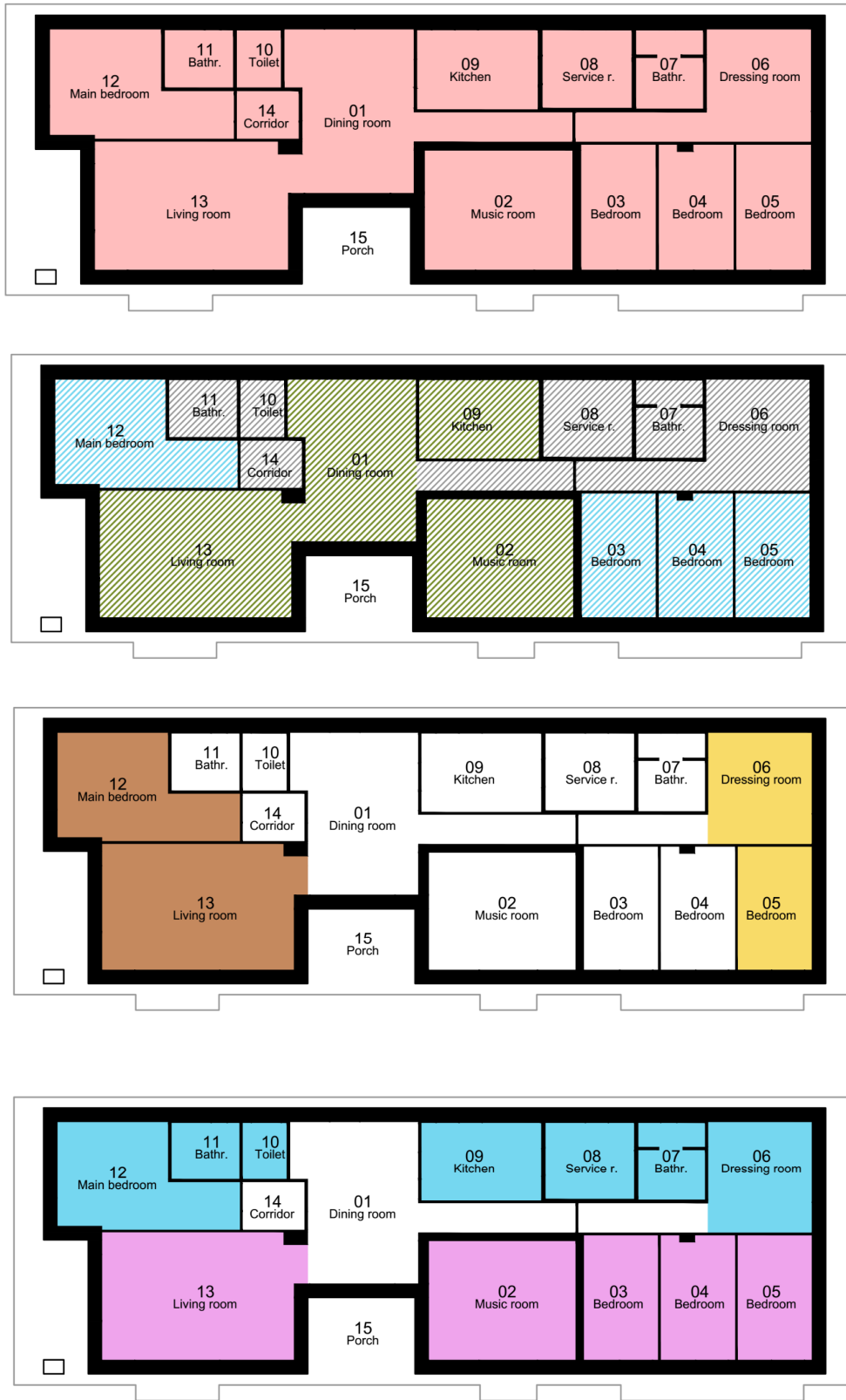
Figure 3.31. Definition of thermal zones in the case study: house average, grouped by activities, West-East sides and North-South sides (from top to bottom).
