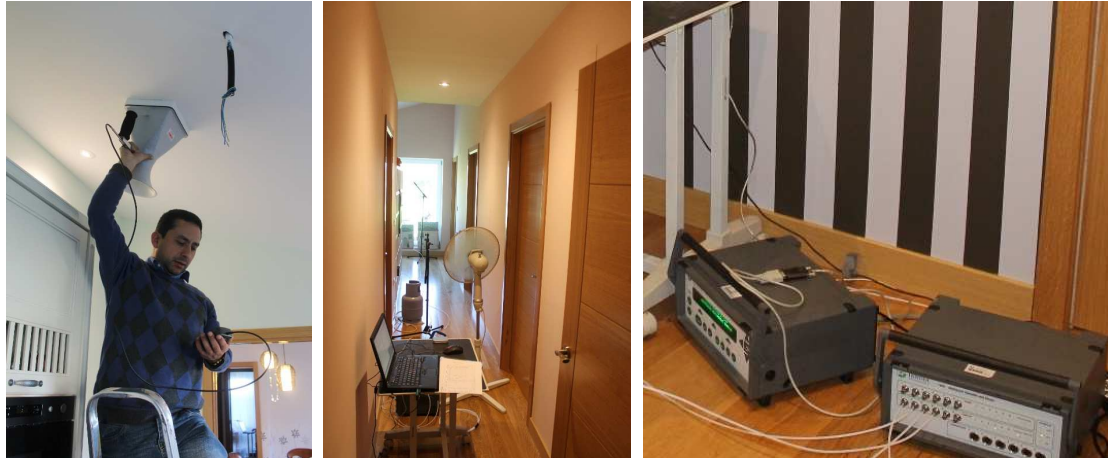
Figure 3.7: Ventilation verification done with different procedures, with an air flow meter (left) and the tracer gas method (centre), gas analysis equipment (right).
