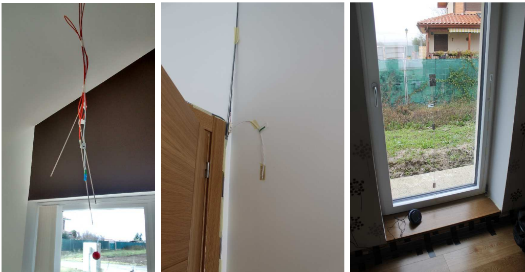
Figure 3.19. Pt100 and RH sensors for living room air (left), surface temperature in column (centre) and surface temperature in the glazing and frame of a window in dressing room (right).
