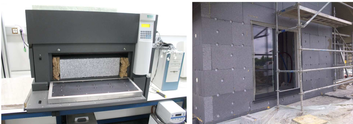
Figure 3.9. Heat flow meter (left) and detail of the EPS installation on facades (right).
