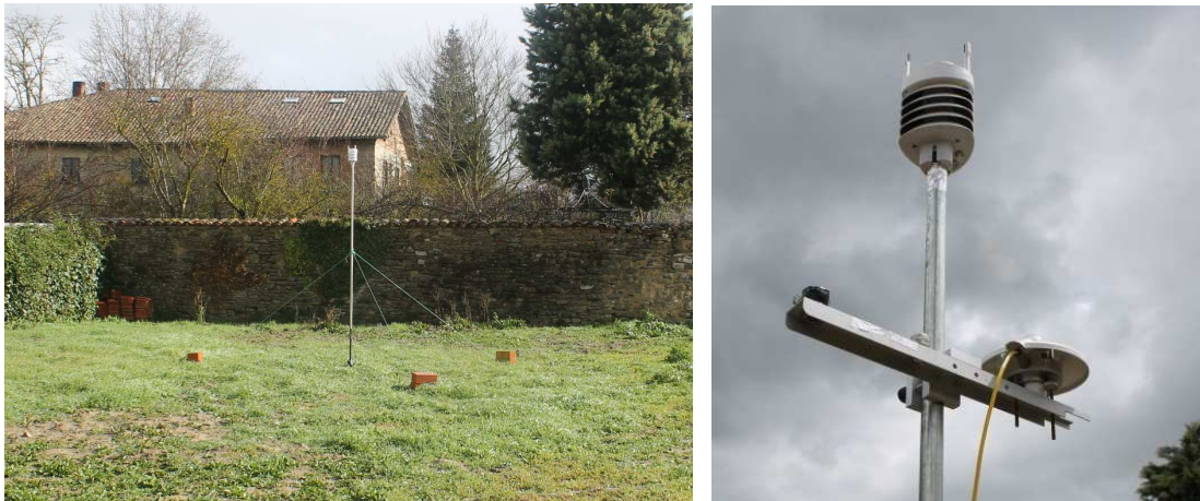
Figure 3.22. Meteorological station location and integration of solar radiation meter on-site.
