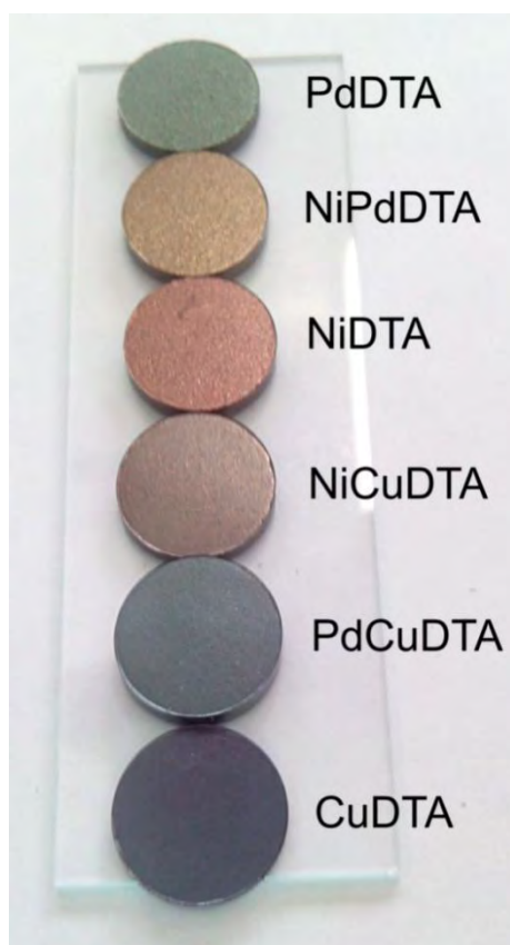
Figure S6.6. Image of MOXs pressed into pellets.
