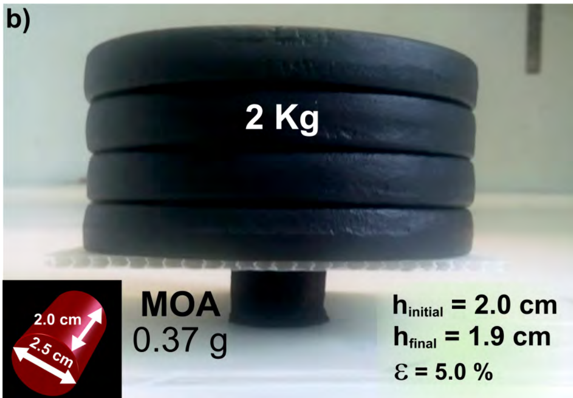
Figure 6. a) MOG (44 g) and b) MOA (0.37 g) monoliths holding up 2 kg of dumbbell weights.
