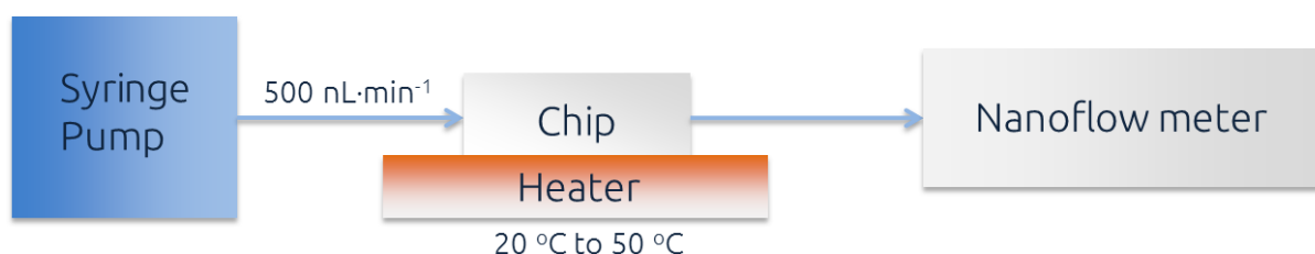
Scheme 2. Setup used for the characterization of DI water flow through the chip.
