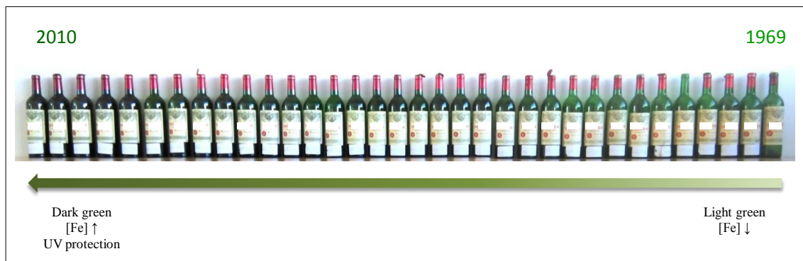
Figure 12 Change of the intensity of green color from the ancient bottles (light green) to newest bottles (dark green)
