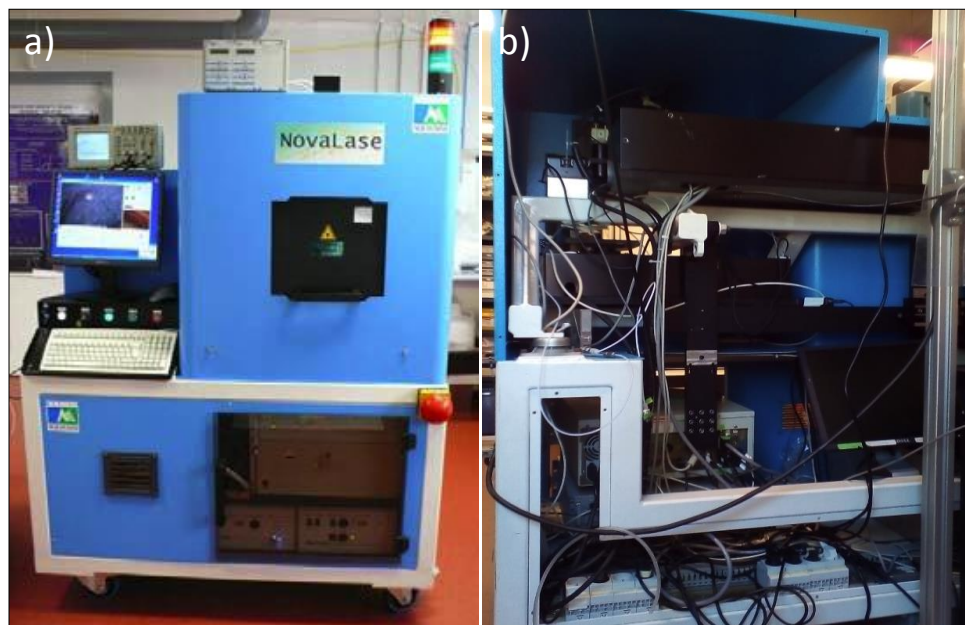
Figure 15 Front and back views of ALFAMET laser ablation device.
