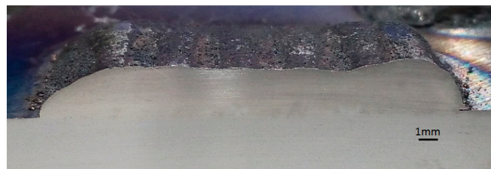
Figure 7. Macrograph of a cross section following the Zig Zag strategy.
