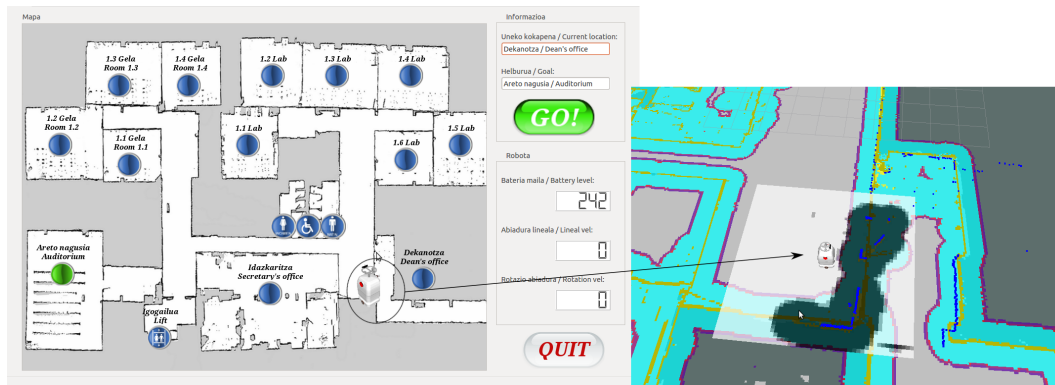
Figure 1. Kbot's navigation interaction window and the current local costmap in RVIZ
