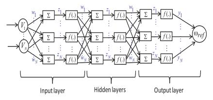
Figure 4. Layout of feed-forward neural network.
