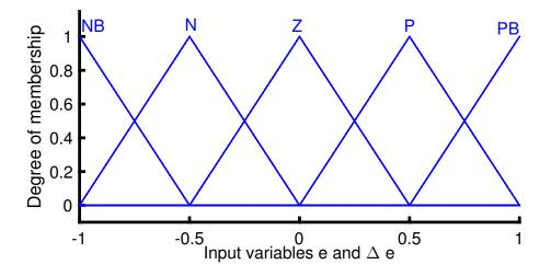
**Figure 8.** Membership functions for inputs *e* and  $\Delta e$ .
