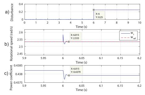
**Figure 25.** Disturbance rejection at t = 6 s. (a) disturbance occurrence; (b) zoom-in rotational speed versus time; (c) zoom-in power coefficient response.
