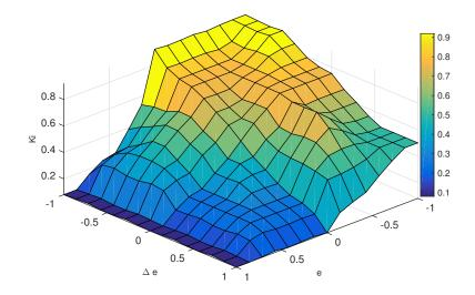
**Figure 11.** Fuzzy surface for *K<sub>i</sub>* gain.
