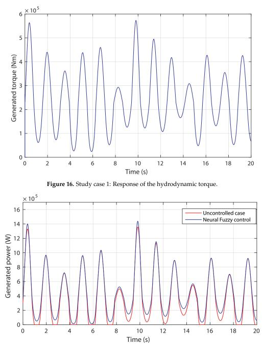
Figure 17. Study case 1: Generated turbine's power curve.
