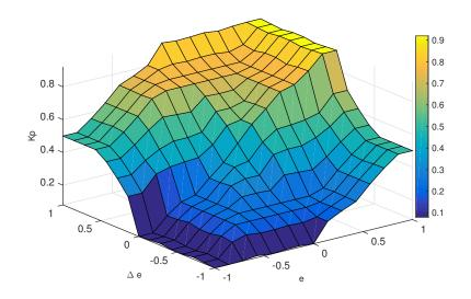
**Figure 10.** Fuzzy surface for *K*<sub>*p*</sub> gain.
