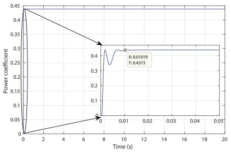
Figure 14. Study case 1: Power coefficient response.
