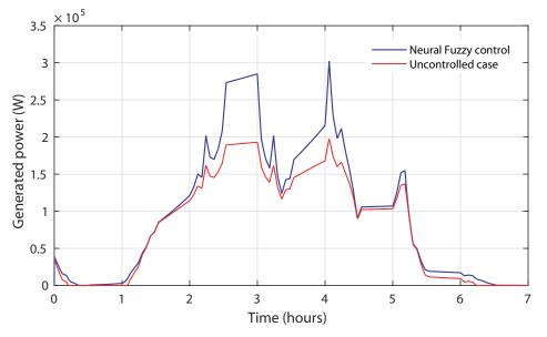
Figure 22. Study case 2: Generated turbine power curve.
