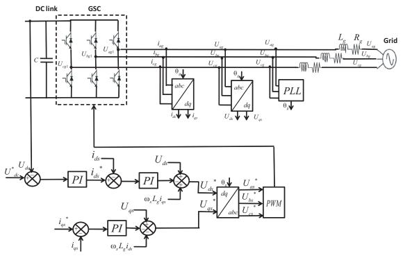
Figure 12. Block control scheme for the GSC component.
