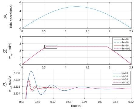
**Figure 5.** Control performances: (a) tidal speed input; (b) response of the reference rotational speed for different number of neurons; (c) zoom into the reference rotational speed variation for 0.07 s.
