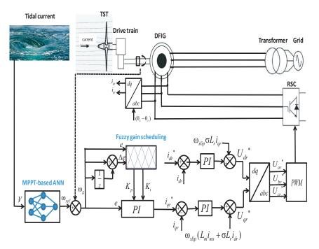
Figure 7. Control scheme of the RSC component.
