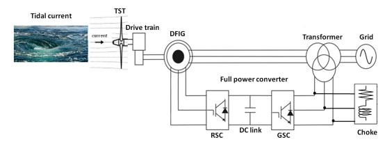
Figure 1. Tidal stream generator global scheme.
