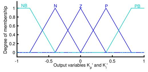
**Figure 9.** Membership functions for outputs  $K'_v$  and  $K'_i$ .
